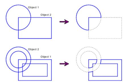
Note that the order in which the objects are identified is important. The last identified object is always "subtracted" from the object identified first.
