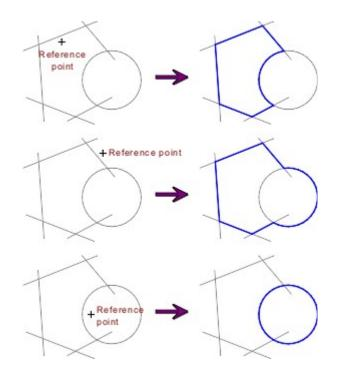
The effect of the reference point can be explained (simply) as follows: Imagine emptying a can of paint at the reference point. The paint spreads out in all directions until it reaches an object. The result is one area which is covered in paint, and one area which is not. The boundary between these two areas is the outline of the newly-generated surface.
