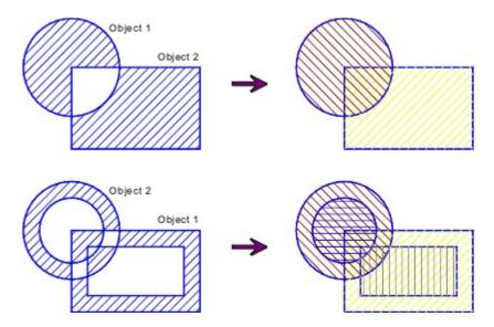
The areas of the objects which are shown hatched, are hatched or filled when the corresponding object is hatched or filled.
