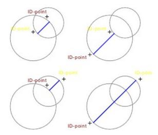
After determining the distance to be measured, the position of the dimension line and dimension text must be specified. To do this, several points have to be entered. How many, and which, points have to be
