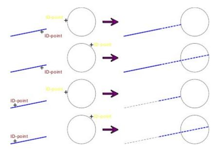
Note a basic rule for trimming: The object changes, wherever it is clicked on.
