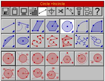
Choosing a command can follow the same procedure as using the text menus. Firstly, the menu is chosen from the upper area ; the menu entries and submenus from that menu appear in the central area. Choosing a menu entry carries out that command, or in the case of a submenu entry, the commands from the submenu appear in the lower arrea.
