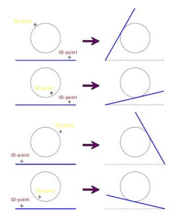
If the trim object is a circle or ellipse part, then the arc end angle closer to the ID point is changed (see graphic).
