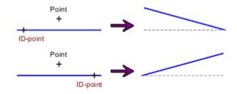
If the trim object is a circle or ellipse part, then the angle at the end of the arc closer to the ID point is altered (see graphic).
