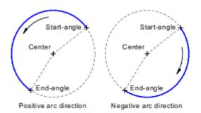
The appearance of the circular arc is shown during input, and changes if the current arc direction is changed.
