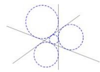
They are presented so that a choice can be made. To do this, a small dialog appears at the bottom of the screen from which the correct geometry circle can be chosen. Only one circle can be chosen at any one time.
