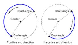
The eventual appearance of the reference circle part is shown during entry, and changes if the arc direction is changed during entry.
