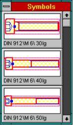
Left-clicking on a button allows the Symbol associated with that button to be placed in the drawing. It hangs from the crosshair and drops into the drawing at the position of the crosshair when the left mouse button is clicked again. This operation can be repeated until the *right* mouse button is clicked, ending the command sequence.
