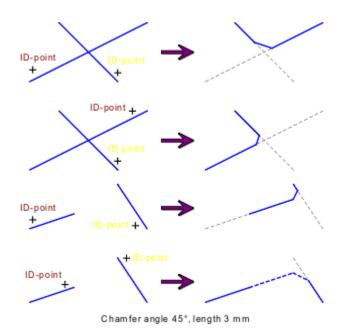
Note a basic rule for trimming: The object changes, wherever it is clicked on.
