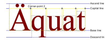
Optionally, specific coordinates can be entered. To do this, press the F8 key or ENTER. Absolute, relative or polar coordinates can now be entered. Relative coordinates relate to the first corner point. For further information on coordinate entry, see <u>Function Keys>Direct Input (F8)</u>.
