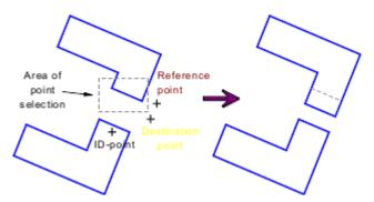
**Note:** The duplicate function does not work with this command, i.e. the objects themselves will be changed. If a copy is required, it must be done before carrying out the command.
