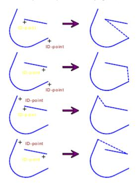
If the duplicate function was active while selecting the second object (e.g. because the CTRL key was held down), the identified objects remain intact. Otherwise they are deleted and only the new, extended curve remains.
