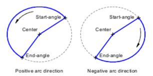
The later appearance of the elliptical sector is shown during entry and changes immediately if the current arc direction is changed during entry.
