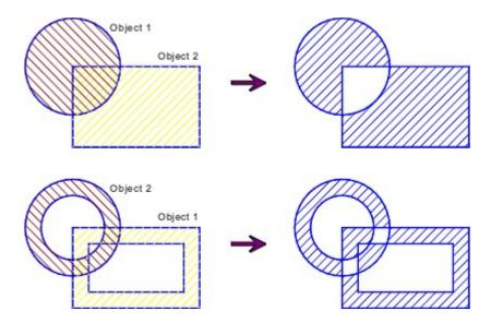
The areas of the objects shown hatched are hatched or filled if the relevant object is hatched or filled. The effects of this combination can be expressed as: (Object 1 - Object 2)  $\times$  (Object 2 - Object 1).
