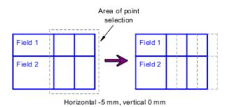
**Note:** The duplicate function does not work with this command, i.e. the objects themselves will be changed. If a copy is required, it must be done before carrying out the command.
