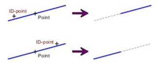
Note this basic rule for trimming: the object is always changed where it is clicked on.
