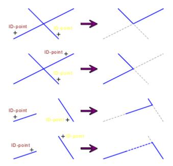
Note a basic rule for trimming: The object changes, wherever it is clicked on.
