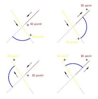
The position of the ID point with reference to each leg shows which angle is measured.
